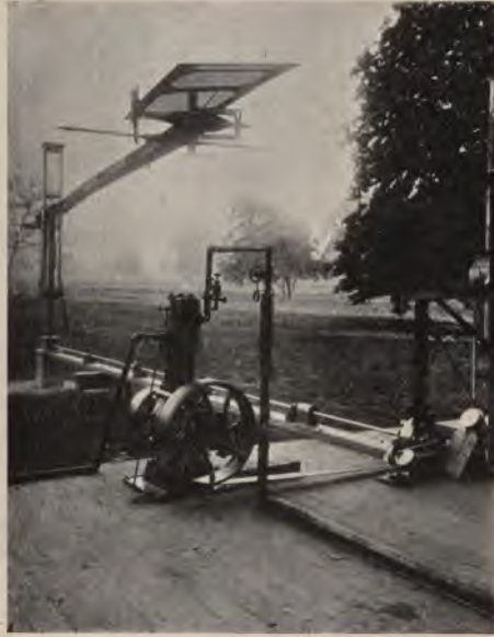
Fig. 34.—The rotating arm of the machine with a screw and aeroplane attached.
